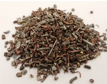
Metals are recovered from the final remaining automotive shredder residue. Gold, silver, copper and palladium are recovered in the form of concentrated precious metal residue.
