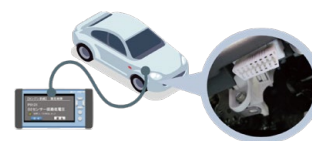
Inspection of an automobile using the USS on-board diagnostics system
