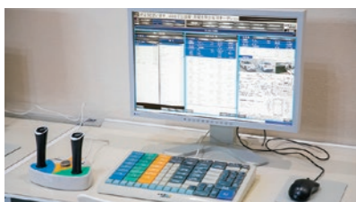
Dedicated satellite TV terminal
